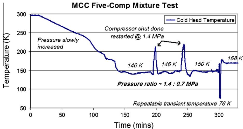
Fig. 5. Cooling test of the MCC using five-component mixed refrigerant. The mixture is precooled to 240 K before sending into the MCC, and the cold head temperature is measured by a thin film Ti thermometer affixed on it.
