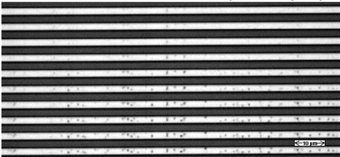
Figure 6. Montage of 10 images during an AC test at 100 Hz of a line fully constrained with SiO<sub>2</sub>. The time series runs from top to bottom. The top image was acquired at 30 s into the test, and the acquisition interval was 10 s. The abrupt change from unvoided to voided is clearly shown.
