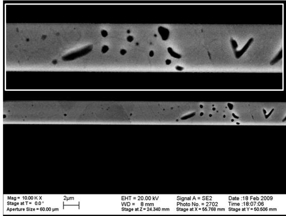
Figure 2. SEM micrograph of a constrained copper line after electrical testing under sinusoidal excitation and removal of the dielectric covering the specimen. This specimen was tested under sinusoidal AC at a peak current density of approximately  $14 \text{ MA/cm}^2$ ; it self-heated to a temperature of  $396 \text{ }^\circ\text{C}$  and had a lifetime of 1497 s. Note the round and elongated void types. Inset: Expanded display of the right-hand portion of the image.
