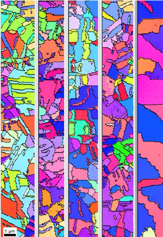
Figure 5. Orientation maps of portions of five damascene copper lines showing the effect of annealing and electrical testing on the grain structure. (a) Grain structure of an as received line. (b) Effect of a 30 h aneal in a vacuum furnace at 300 °C. (c) Orientation map of part of the line shown in Fig. 4 (DC test). (d) Orientation map of a line that received a treatment of 1 h in a vacuum furnace at 420 °C. (e) Orientation map of part of the line shown in Fig. 2 (AC test).
