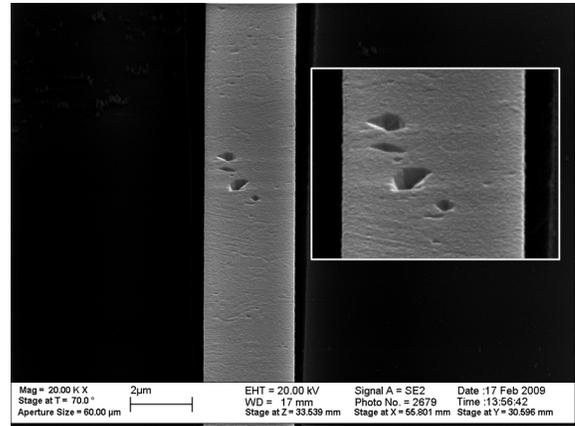
Figure 4. SEM micrograph of a constrained copper line, after electrical testing under DC and removal of the dielectric covering the specimen. It was tested under DC at a current density of approximately  $15 \text{ MA/cm}^2$ ; it self-heated to a temperature of  $413 \text{ }^\circ\text{C}$  above ambient and had a lifetime of 326 s. Inset: region of specimen with voids. Note the faceted void shapes.
