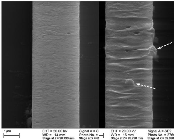
Figure 3. SEM micrograph of copper lines with thin constraint. Left: untested. Right: tested at a peak AC current density of  $13 \text{ MA/cm}^2$ . The cyclic temperature range was  $262 \text{ }^\circ\text{C}$  and the lifetime was 2645 s. The prominences near the lower center and upper right in the tested line (arrows) are copper oxide. The bright horizontal contours indicate topographic features (ridges or grooves). Note the voids.
