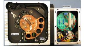
**Figure 1.** Picture of the single-element Si photodiode based colorimeter.
