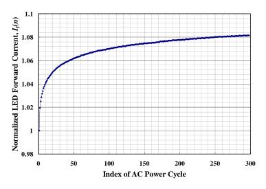
Figure 5. A heating curve of an AC LED.
