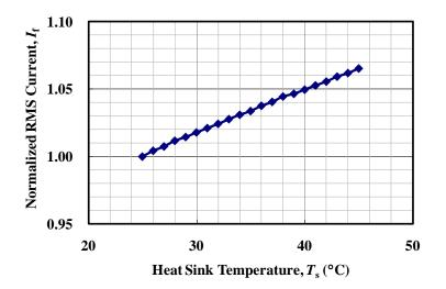
Figure 4. Relationship between the LED RMS forward current,  $I_{\rm f}$ , and the heat sink temperature,  $T_{\rm i}$
