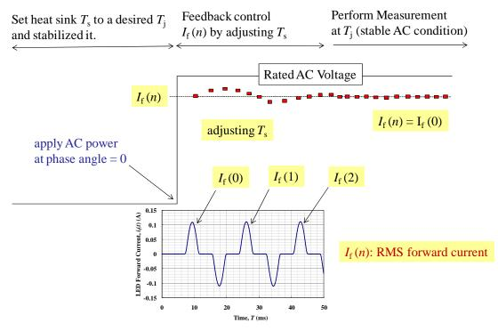
Figure 3. Principle of the simple method for measurement of AC LEDs
