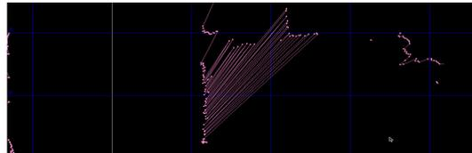
**Figure 10: LMS1 data scanning both a fence and obstacles on the other side of the fence.**
