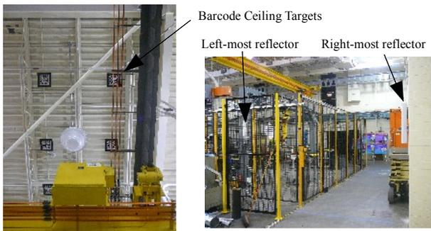
**Figure 8: (left) Crane electrical bars partially occluding the ceiling-mounted 2D bar code targets of the CamPos system; (right) clear view of the right-most reflector of the SLPS system and partially occluded view of the left-most reflector by a robot cage**
