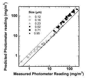
Fig. 3. Comparison of predicted photometer readings to measured readings for DOP aerosols. The lines bound a <u>+</u> 33 % spread between the measured and predicted values.
