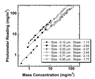
Fig. 2. Mass concentration versus photometer reading for DOP aerosols.
