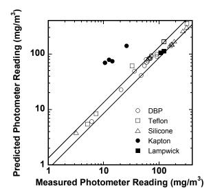
Fig. 4. Comparison of predicted photometer readings to measured readings for SAME experiment smokes. Most predictions fall within a range of <u>+</u> 25 % deviation from measured with the notable exception of Kapton.
