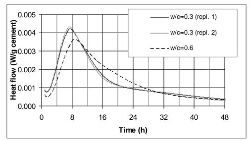
Fig. 4– Isothermal calorimetry curves for Type II/V cement pastes prepared at two different w/c. Results for two replicate specimens for the w/c = 0.3 cement paste are shown to provide an indication of typical variability; for heat flow, 1 W/g = 1548 BTU/(h·lb).
