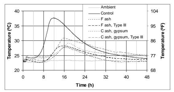
Fig. 2– Semi-adiabatic temperature rise curves for mortars (w/cm = 0.3) without (Control) and with 50 % fly ash replacement for cement. The type of cement (Type III vs. the control Type II/V) is a secondary variable as indicated in the legend.
