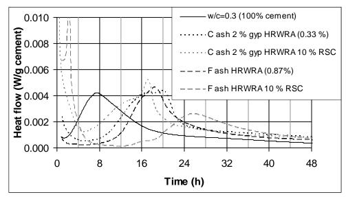
Fig. 12– Isothermal calorimetry curves for Type II/V cement/fly ash pastes prepared with and without the rapid set cement; for heat flow, 1 W/g = 1548 BTU/(h·lb).
