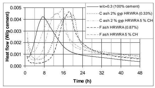
Fig. 10– Isothermal calorimetry curves for Type II/V cement/fly ash pastes prepared with and without 5 % calcium hydroxide additions (all dosages by mass percent of total solids); for heat flow, 1 W/g = 1548 BTU/(h·lb).
