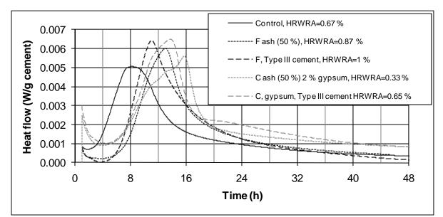
Fig. 1– Isothermal calorimetry curves for mortars (w/cm = 0.3) with and without 50 % fly ash replacement for cement. HRWRA addition levels indicated in the legend are per unit mass of cementitious material (cement + fly ash + gypsum). The type of cement (Type III vs. the control Type II/V) is a secondary variable as indicated in the legend; for heat flow, 1 W/g = 1548 BTU/(h·lb).
