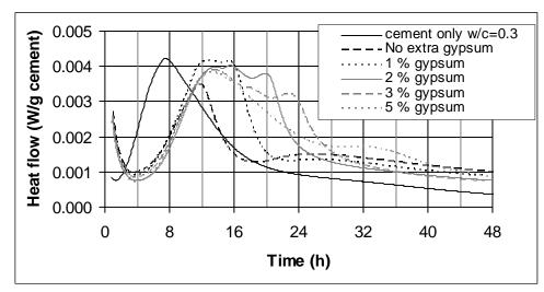
Fig. 5– Isothermal calorimetry curves for 50:50 Type II/V cement/class C fly ash pastes prepared with various levels of calcium sulfate dihydrate additions; for heat flow, 1 W/g = 1548 BTU/(h·lb).
