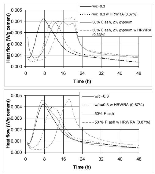
Fig. 6– Isothermal calorimetry curves for 50:50 Type II/V cement/fly ash pastes prepared with and without HRWRA for class C (top) and class F (bottom) ash. HRWRA addition levels indicated in the legend are per unit mass of cementitious material (cement + fly ash + gypsum); for heat flow, 1 W/g = 1548 BTU/(h·lb).
