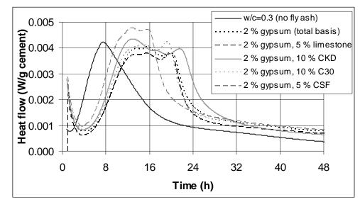
Fig. 7– Isothermal calorimetry curves for 50:50 Type II/V cement/class C fly ash pastes prepared with various powder additions (all additional powder dosages by mass percent of total solids, but gypsum dosage is per unit mass cement + fly ash); for heat flow, 1 W/g = 1548 BTU/(h·lb).
