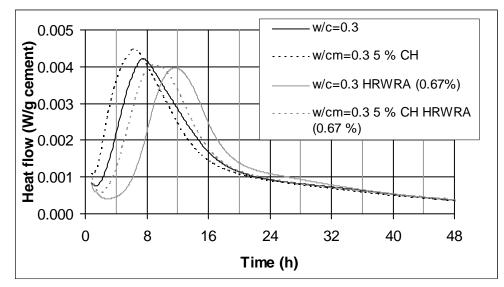
Fig. 9– Isothermal calorimetry curves for Type II/V cement pastes prepared with calcium hydroxide and/or HRWRA additions (all dosages by mass percent of total solids); for heat flow, 1 W/g = 1548 BTU/(h·lb).
