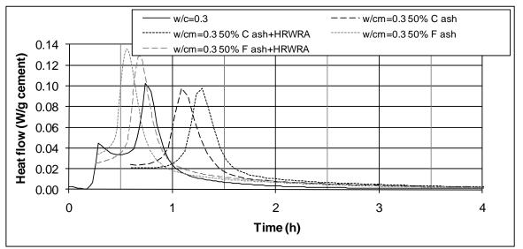
Fig. 11– Isothermal calorimetry curves for rapid set cement/fly ash pastes prepared with and without the HRWRA. HRWRA was added at a dosage of 0.33 % of total solids by mass; for heat flow, 1 W/g = 1548 BTU/(h·lb).
