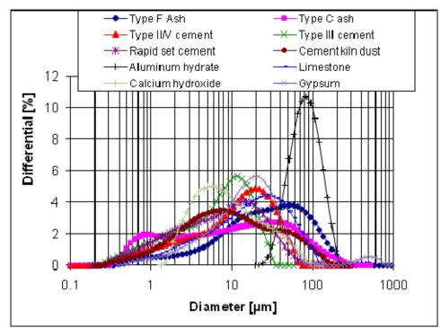
Fig. 3– Measured PSDs for the powders employed in the present study. The shown results are the average of six individual measurements and the error bars (one standard deviation) would fall within the size of the shown symbols. (One micrometer is equivalent to  $3.9 \times 10^{-5}$  in.)
