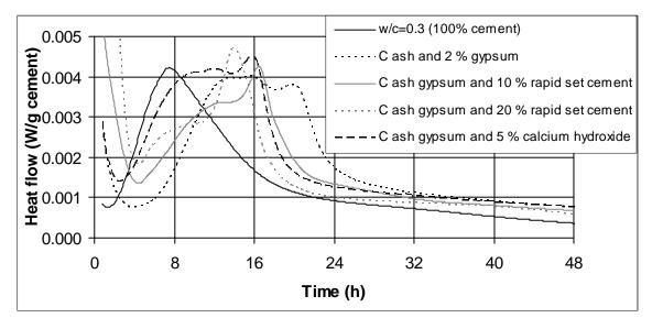
Fig. 8– Isothermal calorimetry curves for 50:50 Type II/V cement/class C fly ash pastes prepared with calcium hydroxide or rapid set cement additions (all additional powder dosages by mass percent of total solids); for heat flow, 1 W/g = 1548 BTU/(h·lb).
