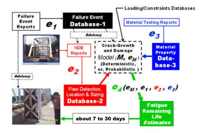
Figure 1 A conceptual representation (after Fong and Marcal [2] and Fong, Ranson, Vachon, and Marcal [3]) of the information flow plus the uncertainties and potential errors associated with and inherent in (1) Failure Event Database-1 (Uncertainty-1, or, e<sub>1</sub>), (2) Flaw Detection, Location & Sizing Database-2 (Uncertainty-2, or, e<sub>2</sub>), (3) Material Property Database-3 (Uncertainty-3, or, e<sub>3</sub>), (4) Deterministic or Probabilistic Damage Models
