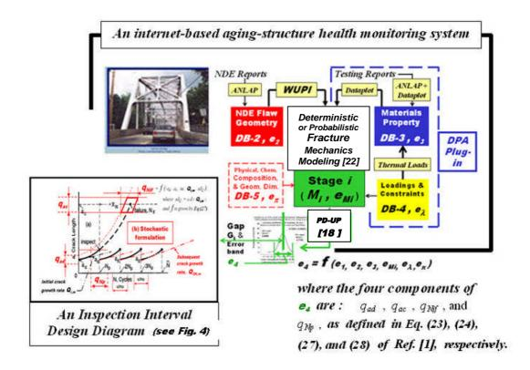
Figure 8 A schematic design of the internet-based aging-structure health monitoring system involving the use of ANLAP [8, 9](to manage  $e_1$ , WUPI [1] to manage  $e_2$ , DPA [21] to manage  $e_3$ , and PD-UP [18] to manage  $e_M$  for a stochastic fracture mechanics-based crack growth model [22]. Note that in this web-based computational exercise, the five source uncertainties,
