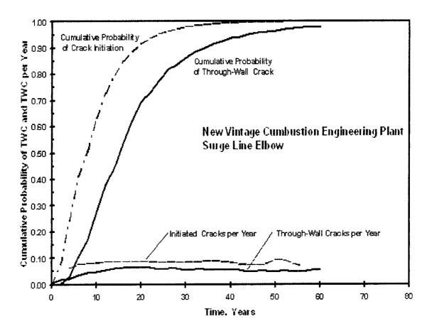
Figure 2 Calculated Probabilities of Crack Initiation and Through-Wall Crack for the Surge-Line Elbow of the Newer Vintage Combustion Engineering Plant (after Khaleel, Simonen, Phan, Harris, and Dedhia [5]).
