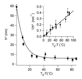
**Fig. 5.** Free surface layer thickness as determined from the bilayer model is strongly correlated with quench depth into the glass for  $(\bullet)$  PS and  $(\blacksquare)$  poly(n-alkyl meth-acrylate)s. The data for the polymethacrylates are taken from [35]. The dashed lines are exponential and linear (inset) fits of the data, and the error bars represent one standard deviation of the data, which is taken as the experimental uncertainty of the measurement.
