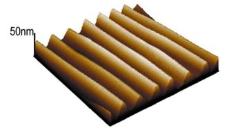
Fig. 2. AFM images of wrinkled films of 25 nm thick 990 kg/mol PS film. Scan size is 7.5  $\mu$ m  $\times$  7.5  $\mu$ m and the height scale of the micrograph is 50 nm as shown.
