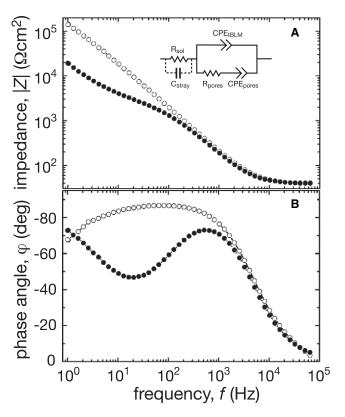
FIGURE 1 EIS spectra of a tBLM before and after  $\alpha$ -HL reconstitution. The Bode plots (*A*) and phase angles (*B*) were measured with tBLMs in 0.1 M NaCl, 5 mM phosphate buffer at pH 7.5 before (*open circles*) and 2 h after the addition of  $\alpha$ -HL to a final concentration of 50 nM (*solid circles*). The temperature was  $(21 \pm 1)^{\circ}$ C. The data were normalized with respect to the membrane surface area. (*Inset*) Equivalent model circuit for the tBLM.
