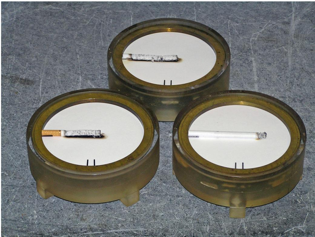
**Figure 1. Photograph of Typical Results of Determinations using ASTM E 2187-04. Top: full-length burn of a non-filter cigarette; Left: full-length burn of a filter cigarette; Right: ceased burning of a less fire-prone cigarette.**
