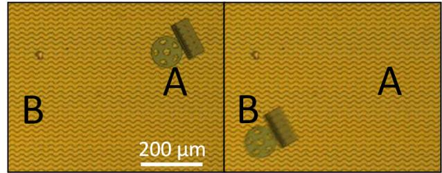
**Figure 1** A sequence of two images showing an electrostatic microrobot moving a silicon disc (soccer ball) from point A to point B (elapsed time  $\approx 3.5$  s)
