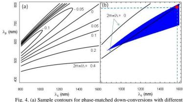
groups of pump and signal wavelengths, each group has a certain spatial harmonic frequency. (b)Shaded spectral region of interest. The red dot corresponds to the phase-matched down-conversion at  $\lambda_p = 764$  nm,  $\lambda_s = 1550$  nm and  $\lambda_i = 1506$  nm. See text for detail.
