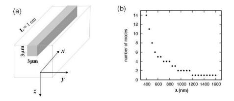
Fig. 1. (a) Schema for a KTP crystal containing a waveguide. The waveguide dimensions and crystal axes are labeled. (b) Number of bound modes in the waveguide with polarization along z-axis.
