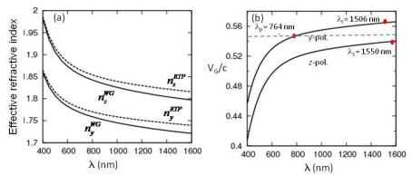
Fig. 3. (a) Effective refractive index of y- or z- polarized light beam propagating in bulk RTP and waveguide (WG). (b) Group velocity of y- or z- polarized optical modes in the waveguide. A selected group of wavelengths with group velocities satisfying Eq. (10) is shown as the red dots.
