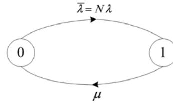
Fig. 1. Markov process model for channel occupancy  $\{X(t); t \geq 0\}$ .
