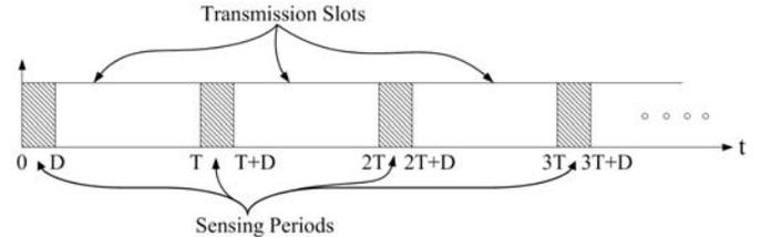
Fig. 2. The SU behaves in a periodic manner. It senses the channel for  $D$  seconds and then it may use it for  $W = T - D$  seconds or wait for  $W$  seconds.
