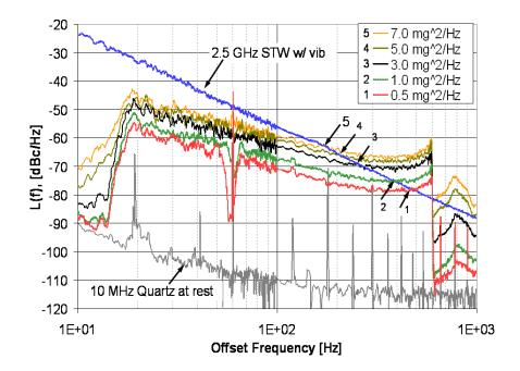
Figure 6. PM noise of free-running oscillators under vibration along the z-axis. Vibration sensitivity of each oscillator causes the optimum PLL BW at  $f_{cross}$  shown by arrows to depend on vibration level. A random vibration is applied between 20 Hz  $\leq f_v \leq$  10 kHz.
