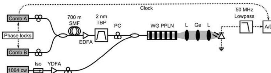
Fig. 1: DFG comb setup. Combs A and B are each Er-fiber-laser frequency combs that are phase-locked together with sub-radian phase noise. Their output is stretched, amplified, filtered, and then converted to around 3.375  $\mu\text{m}$  in a ridge waveguide PPLN. The 1064 nm laser is a cw fiber laser. EDFA: Erbium-doped fiber amplifier, SMF: single-mode fiber, TBP: tunable bandpass, PC: polarization control, L: CaF lens, Ge: Germanium filter.
