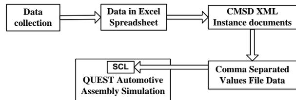
Figure 2: Process data input flow diagram
