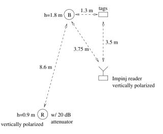
Fig. 8. RFID reader illuminating communications antenna
