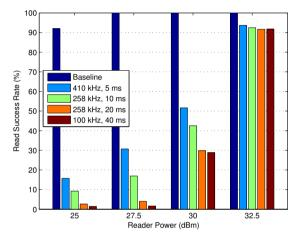
Fig. 7. RFID read success rate vs. reader power by *interference profile*; 30 dBm interferer; single tag one-half wavelength from aluminum plate
