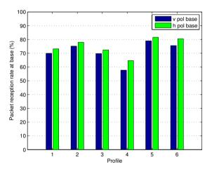
Fig. 10. Packet reception rate at base vs profile, by base antenna polarization; 32.5 dBm reader; vertically polarized reader antenna
