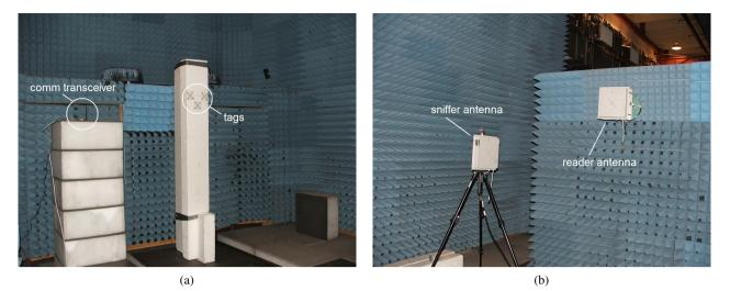
Fig. 3. (a) Communications device (left) and RFID tags; (b) Sniffer and RFID reader (right) antennas
