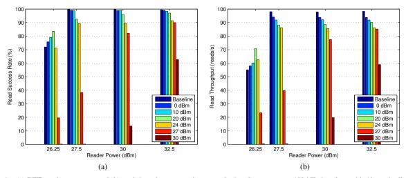
Fig. 4. (a) RFID read success rate and (b) read throughput vs. reader power, by interference power; 100 kHz interferer with 40 ms dwell time
