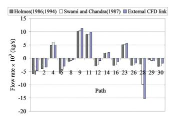
Figure 6. Comparison of calculated infiltration rates using wind pressure coefficients predicted by the external CFD link, measured data from Holmes (1986, 1994), and surface-averaged data from Swami (1987) when the wind is out of the west (270°).
