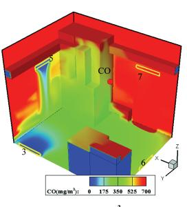
Figure 7. Distribution of CO concentration (mg/m<sup>3</sup>) in utility room at end of 2 h simulation time (1 mg/m<sup>3</sup>  $\approx$  9.9 × 10<sup>-7</sup> oz/ft<sup>3</sup>).
