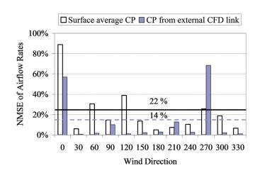
Figure 5. NMSE of predicted airflow rates under different wind directions using averaged wind pressure coefficients (Swami and Chandra 1987) and predicted values from the external CFD link.
