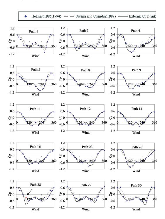
Figure 4. Comparison of calculated profiles of wind pressure coefficient by the external CFD link, measured data at each airflow path (Holmes 1986, 1994), and average data for each building surface (Swami and Chandra 1987) of the house.
