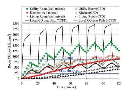
Figure 8. Comparison of CO levels in utility room, kitchen, and living room of the house with and without CFD simulations.
