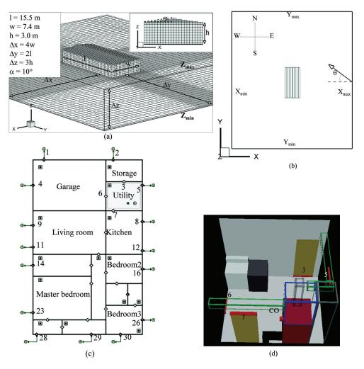
Figure 3. (a) CFD mesh, (b) plan view of building in CFD, (c) CONTAM zone configuration with shaded zone of the utility room, and (d) internal view of utility room in CFD.
