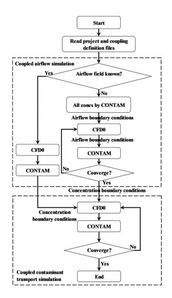
Figure 2. Schematic of embedding a CFD zone in the CONTAM airflow network for simulations at steady state in CONTAM 3.0.
