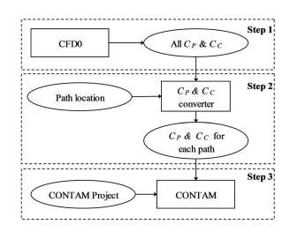
Figure 1. Schematic of link between CONTAM and CFD0 for building external airflow and contaminant transport simulations.
