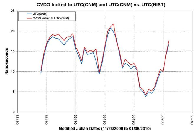
FIG. 6. (Color online) Phase comparison between UTC(CNM) time scale and CVDO locked to UTC(CNM).
