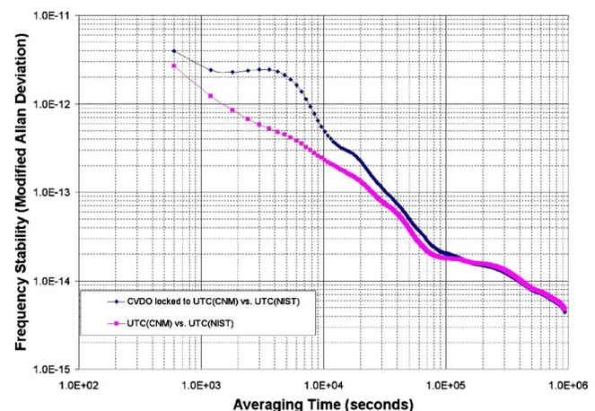
FIG. 7. (Color online) Stability comparison between UTC(CNM) time scale and CVDO locked to UTC(CNM).
