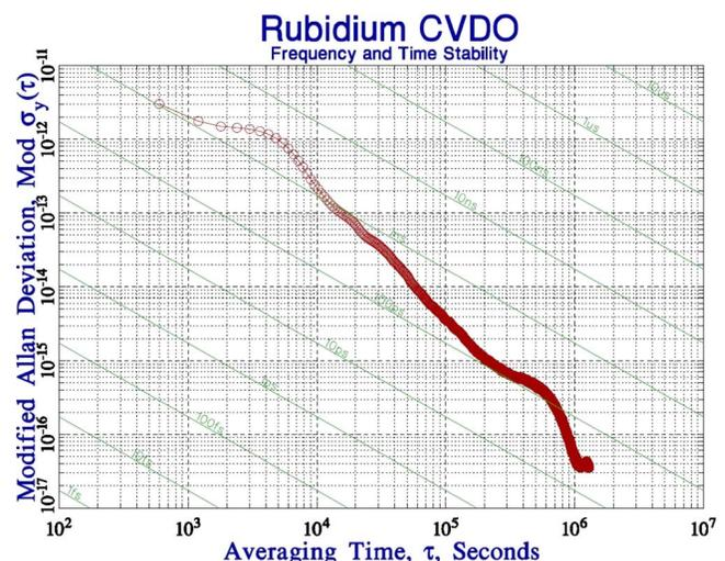
FIG. 4. (Color online) Frequency stability and time stability (diagonal lines) of the rubidium CVDO 1 pulse/s output with respect to UTC(NIST).
