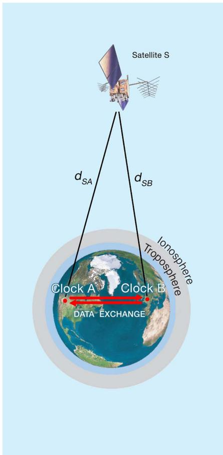
FIG. 1. (Color online) The common-view GPS measurement method.
