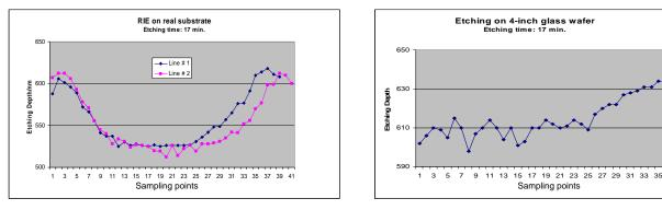
Fig.3 Etching Depth with Sample substrate
