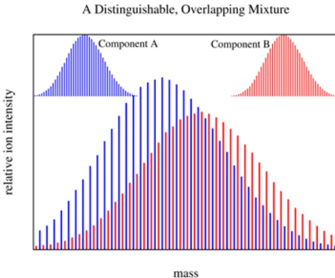
Figure 5— Schematic illustration of a distinguishable but overlapping mixture of two components.
