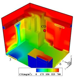
Figure 7Distribution of CO concentration  $(mg/m^3)$  in the utility room at end of the two hour simulation time
