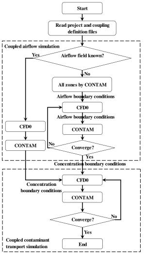
Figure 2 Schematic of embedding a CFD zone within the CONTAM airflow network for simulations at steady state in CONTAM 3.0
