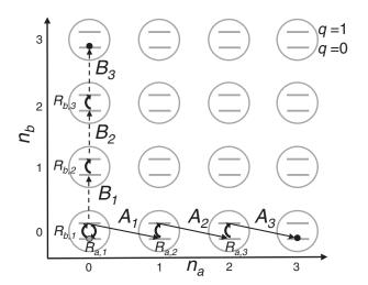
FIG. 3. Algorithm to generate the state  $|\Psi\rangle = |3,0\rangle + |0,3\rangle$  of two coupled resonators. The sequence of operations is detailed in Table I. The horizontal, vertical, and curved transitions are the interactions A, B, and R (see text).
