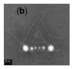
Scanning electron microscope image of a single set of Au nanoparticles assembled onto a DNA origami template. The triangle shows the location of the origami relative to the nanoparticles.
