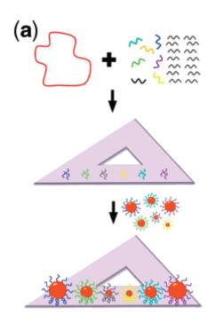
Schematic of the assembly process showing the addition of single-stranded viral DNA and the staple strands, with some specially configured to provide sticky ends for nanoparticle attachment, to form a triangular origami tile with attached, DNA-functionalized Au nanoparticles.
