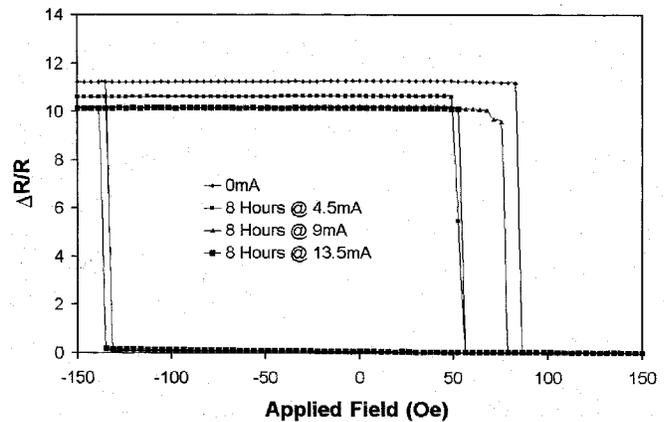
Fig. 6. Magnetoresistive decay of a 1  $\mu$ m device due to sustained current stress while the substrate was maintained at 77°K.
