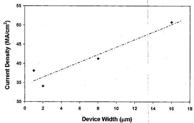
Fig. 4. Current densities that result in device failure for each spin valve stripe width tested.
