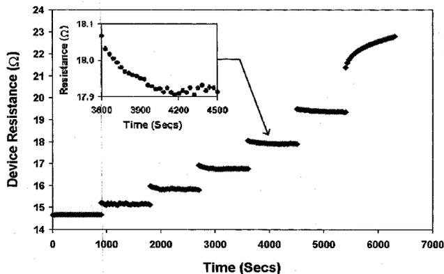
Fig. 3. Device resistance versus time for an increasing applied current (Initial current level =  $2\ \text{mA}$ , increment =  $2\ \text{mA}$ ). The inset is a close-up of the initial resistive increase and subsequent decrease within the  $1\ \mu\text{m}$  device.
