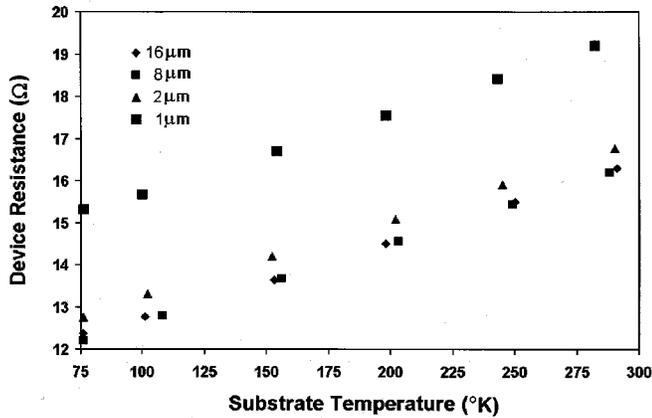
Fig. 2. Device resistance as the substrate was cooled from  $300^{\circ}\text{K}$  to  $77^{\circ}\text{K}$  with an applied magnetic field of  $8\ \text{kA/m}$ .
