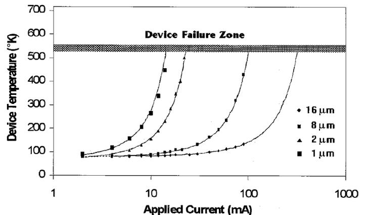
Fig. 5. Internal device temperature as generated by an applied current for each device size tested.
