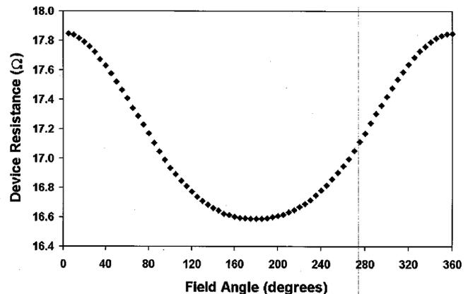
Fig. 1. Determination of the free layer and pinning layer alignment by measuring the magnetoresistance while rotating the device in an 8 kA/m magnetic field.
