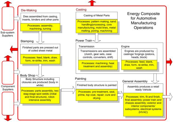
Figure 10 Energy composite for automotive manufacturing operations
