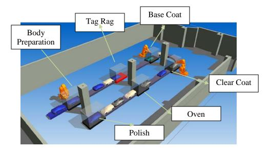
Figure 14 The 3D Simulation model of the paint shop
