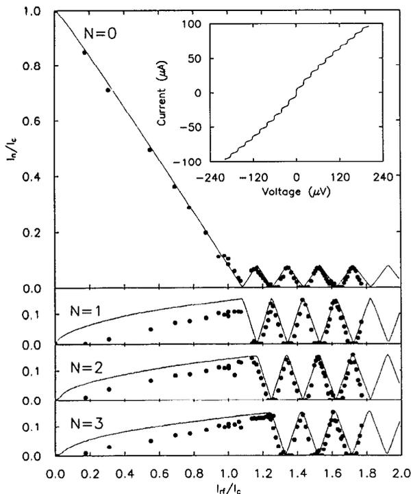
FIG. 4. Step size vs microwave current for the  $N = 0, 1, 2,$  and  $3$  steps. The solid line is from a numerical solution of the RSJ equations with a parallel microwave current source. The inset is the  $I$ - $V$  curve for this microbridge with 7 GHz microwaves applied, showing the constant voltage steps at  $14 \mu\text{V}$  intervals.
