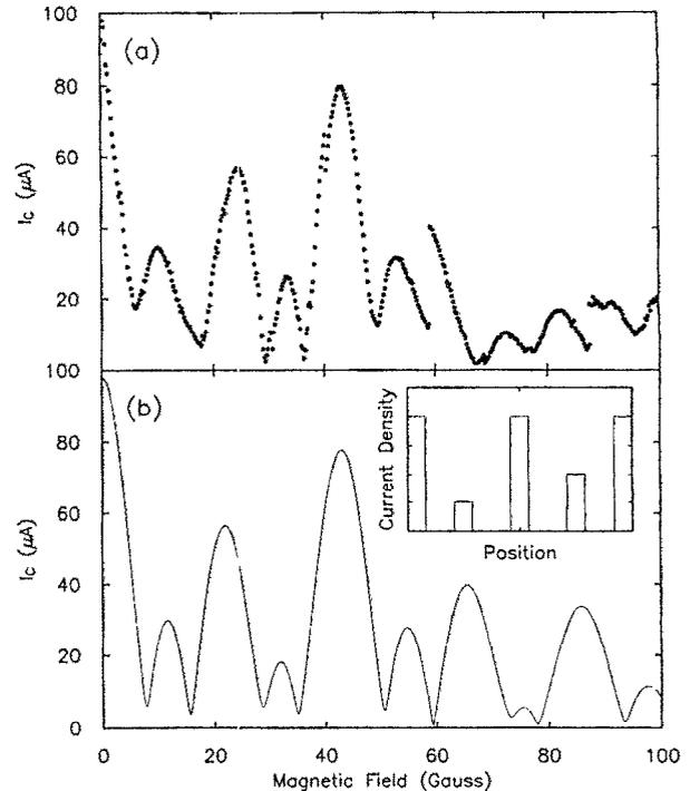
FIG. 2. (a) Critical current vs magnetic field for a typical device exhibiting oscillatory behavior, but the peak heights are uneven and the minima do not quite reach zero. (b) Theoretical behavior of an asymmetric, nonuniform junction showing many of the same features as the real device. The inset is the local critical current vs position used for this simulation.
