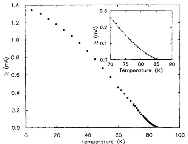
FIG. 3. Critical current vs temperature for a relatively strong high-angle grain boundary weak link. Inset is an expanded view near  $T_C$  with a fit to  $(1 - T/T_C)^{-1.5}$ .
