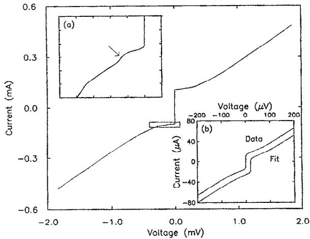
FIG. 1.  $I$ - $V$  curve for typical high-angle grain boundary microbridge at 4.2 K. Inset (a) is an expanded view of the same data, the arrow points to a small deviation from ideal RSJ behavior probably due to supercurrent self-resonant effects. Inset (b) shows data for the same device taken at 60 K and a fit to the RSJ model with noise rounding. The curves are offset for clarity, but when overlaid the fit is essentially exact.
