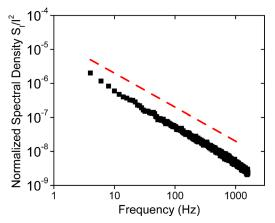
FIG. 3. (Color online) Spectral noise density *S* for a typical single crystal TBDMS transistor ( $V_{DS}$ =-1.0 V,  $V_{GS}$ =-20.0 V). The solid black squares can be fit to  $S \propto f^{-1.01}$  in this case. The dashed line shows a  $S \propto f^{-1}$  behavior to guide the eye.
