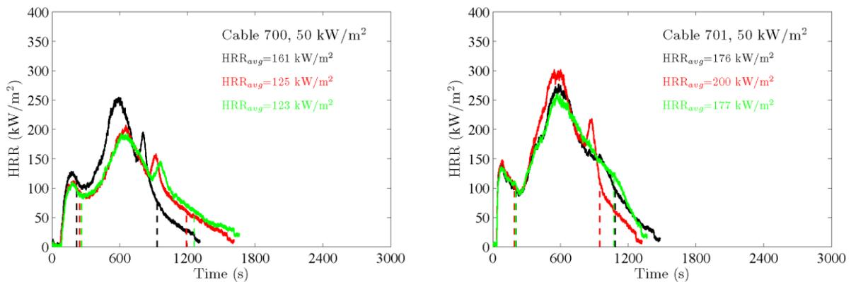
**FIGURE 7. Cone calorimeter results for a thermoset (left) and thermoplastic (right) cables. The heat flux of 50 kW/m<sup>2</sup> represents the power of the cone heater. The HRR values represent the heat released per unit area of sample for the three replicate experiments.**
