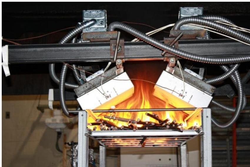
**FIGURE 3. End view of radiant panel apparatus**
