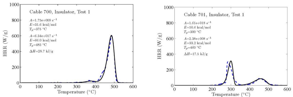
**FIGURE 5. MCC results for a typical thermoset (left) and thermoplastic (right) cable.**
