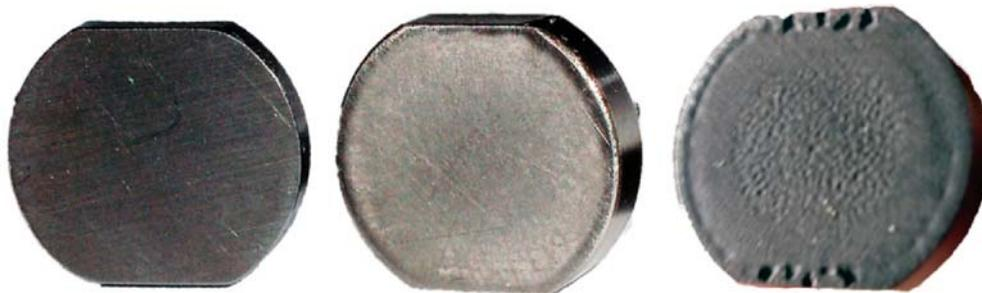
Figure 7. Active surface of removable  $1/2$ -inch flat tips, ranging from pristine (left) to matted (center) to eroded with extensive pitting (right).
