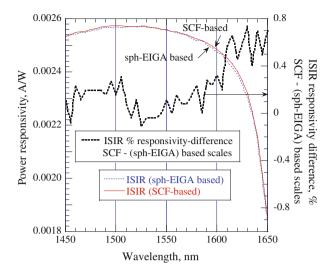
Fig. 3 SCF-determined and SIRCUS tie-points-corrected spectral responsivity of the ISIR
