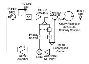
Figure 2. Block diagram of the cavity stabilized oscillator (CSO) at 40 GHz. The 10 GHz DRO is phase-locked to the phase-transfer function of the air-cavity resonance. DBM is double-balanced mixer, ATTEN is attenuator and  $\beta_1$  is input coupling.
