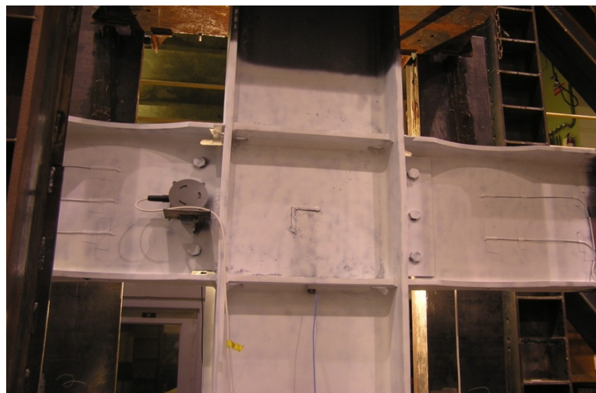
Figure 3–8 Inclinometer attachment to RBS specimen
