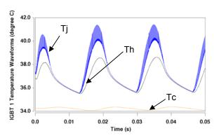
Fig. 14. Temperature waveforms of IGBT1 showing surface Tj, header chip interface Th, and case base-plate interface Tc.
