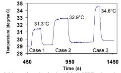
Fig. 9. Measured transient heating of single IGBT under various power conditions
