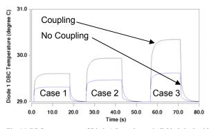
Fig. 16. DBC temperatures of Diode 1 for each case in Table 2, both with and without device-device coupling.
