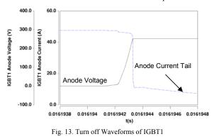
Thus, a large anode-cathode voltage and current exist at the same time, resulting in a large power dissipation and temperature spike at turn-off. Although the power dissipation level is not as high as during the turn-on event, the turn-off switching time is much longer due to the slowly decaying excess carriers in the IGBT base. Thus, the turnoff switching energy  $E_{sw,off}$  indicated in Fig. 12(e) is larger than the turn-on energy.
