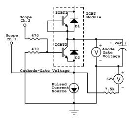
Fig. 6. High Speed IGBT Thermal transient test circuit.
