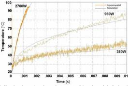
Fig.7. Simulated transient thermal response of 6-pack module for heating of single IGBT under various power conditions with experimental verification using high-speed temperature sensitive parameter measurement.
