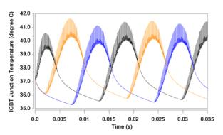
Fig. 11. Simulated three-phase inverter IGBT chip junction temperature waveform for each phase in two 60 Hz cycles of the inverter for the 10.8 kW condition.
