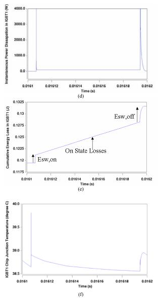
Fig. 12. Simulation results of one 10 kHz switching cycle for the (a) IGBT anode current, (b) current though D2, (c) anode voltage,(d) power dissipation, (e) energy and (f) IGBT chip surface temperature for Case 3.
