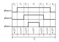
Fig. 5. Space vector modulation diagram timing diagram of the SVM inverter control algorithm.
