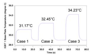
Fig. 15. Base-plate temperatures of IGBT1 for the cases shown in Table 2.
