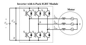
Fig. 2. Circuit diagram of the three-phase inverter motor drive using a six-pack IGBT module.
