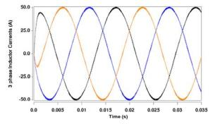
Fig. 10. Simulated three-phase inverter current waveform for each phase in a two 60 Hz cycles of the inverter for the 10.8 kW condition.
