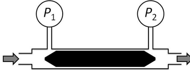
Figure 9. Longitudinal cross section of the annular LFM. The gas flowed through the small gap between concentric cylinders. The tapered end of the inner cylinder reduced turbulence in the gas exiting the gap. The inner cylinder used in the circular segment LFM cylinder had a similar taper.
