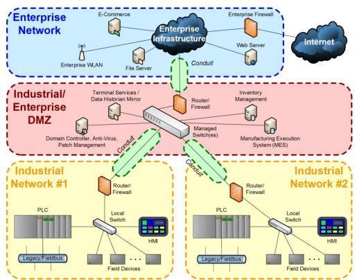
Figure 3 – High-level manufacturing example showing zones and conduits
