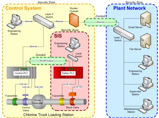
Figure 2 – High-level process-industry example showing zones and conduits
