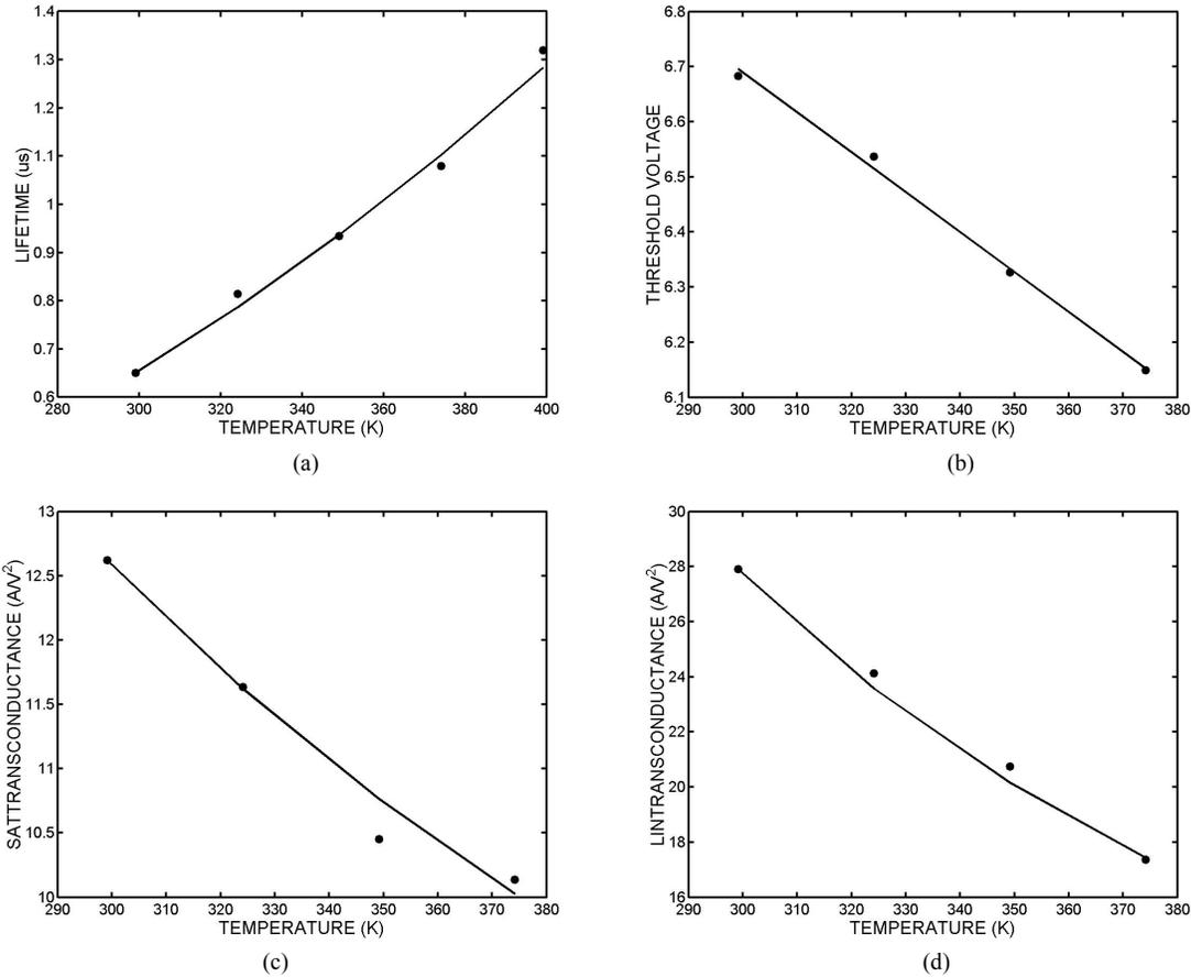
Fig. 1. IGBT temperature dependent model parameters: (a) Lifetime vs. Temperature; (b) Threshold Voltage vs. Temperature; (c) Saturation Transconductance vs. Temperature; and (d) Linear Transconductance vs. Temperature.
