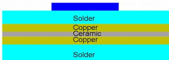
Fig.3 Direct Bonded Copper (DBC) layer structure
