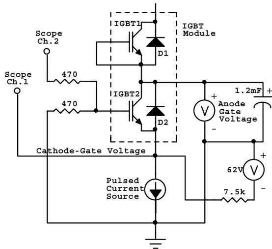
Fig. 7. High Speed IGBT Thermal transient test circuit.
