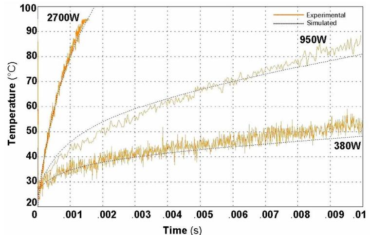
Fig. 8. Transient heating of single IGBT under various power conditions
