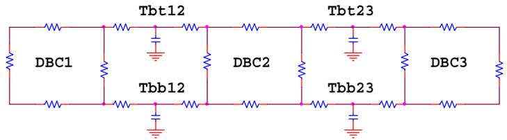
Fig.6 Coupling network of baseplate
