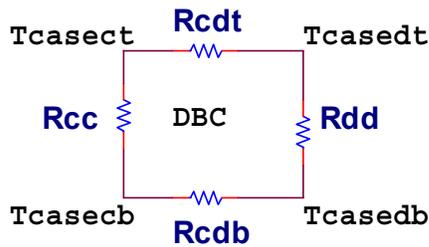
Fig. 5 Coupling network of DBC
