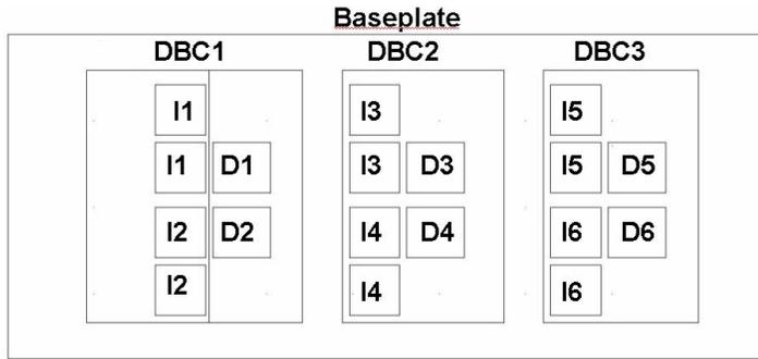
Fig.2 Internal structure of the SEMIKRON power module
