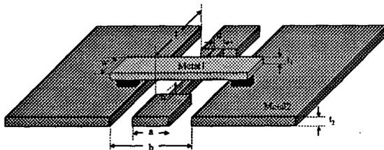
Figure 2: Illustration of a compensated ground equalization section used in BLC. The bridge-like structure is 1<sup>st</sup> metal layer (Metal1). The discontinuities in the signal are symmetric with respect to Metal1. Coplanar transmission is symmetric and realized by using 2<sup>nd</sup> metal layer (Metal2).
