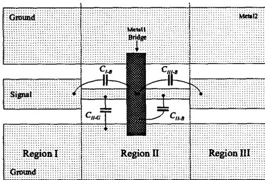
Figure 3: Ground equalizers are modeled with a shunt lumped capacitance  $C_{ge}$ . Although, this quasi-static capacitance is dominated by  $C_{II-B}$  in many cases, if  $l$  is  $< 2w$  then the contributions from  $C_{I-B}$  and  $C_{III-B}$  are substantial. If  $l > 3w$ , on the other hand, then  $C_{II-G}$  should be considered as well.
