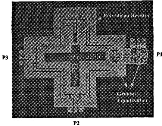
Figure 1: Microphotograph of the micromachined Ka-band branch line coupler.
