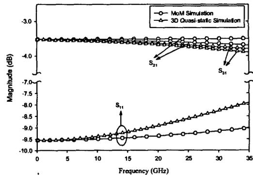
Figure 5: The T-junctions with  $(l,d)=(35,10)$  for  $50 \Omega$  and  $(35,20)$  for  $35 \Omega$  are simulated by using the capacitances from a 3D quasi-static field solver. If these results are compared with 2 $\frac{1}{2}$ D simulation (with zero-thickness strips) results, significant difference at frequencies above 10 GHz is observed.
