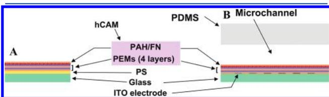
**Figure 2.** Side view of a glass coverslip (A) and a DEP device (B), both with the hCAM deposited on top. The hCAM is comprised of a layer of FN and PAH on top of four layers of polyelectrolytes ((PAH/PSS)<sub>2</sub>), which in turn were deposited onto polystyrene-coated coverslips (A) and ITO electrodes (B). The microchannel is molded in PDMS and reversibly bound onto the device.
