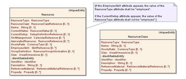
Figure 3 - The Resource and ResourceClass UML Diagram
