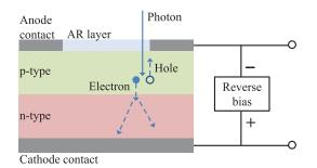
FIG. 7. (Color) A single-photon avalanche photodiode is shown with distinct regions for the photo-absorption and carrier multiplication processes. The voltage is applied to accelerate the electrons toward the multiplication region. A front-illuminated geometry with an antireflection (AR) coating to improve efficiency is illustrated, but back-illuminated designs are also used.
