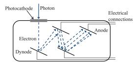
FIG. 6. (Color online) A photomultiplier, the first detector able to sense a single optical photon, is shown schematically with a transmissive photocathode and just 3 dynodes. The photocathode may be designed to have the photoelectrons emitted from its front or back surface and typically 10 dynodes are used.
