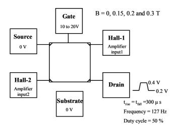
Fig. 2. The 4H-SiC Van der Pauw structure measured, which has an active gate area of 150  $\mu$ m × 150  $\mu$ m. The setup shown here is for the inversion sheet charge density (n<sub>s</sub>) measurement.
