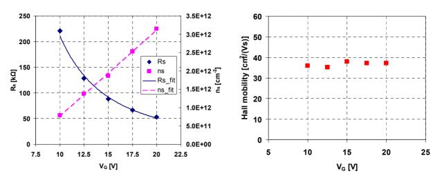
Fig. 5. Sheet resistance and inversion sheet Fig. 6. Hall mobility calculated from Rs and charge density measured at different gate  $n_s$  as a function of gate voltage. voltages.
