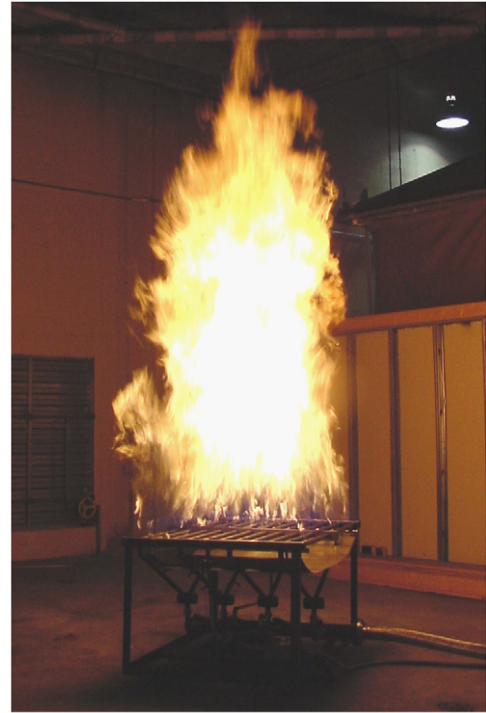
Fig. 1. Photo of a 3 MW fire from the natural gas burner.
