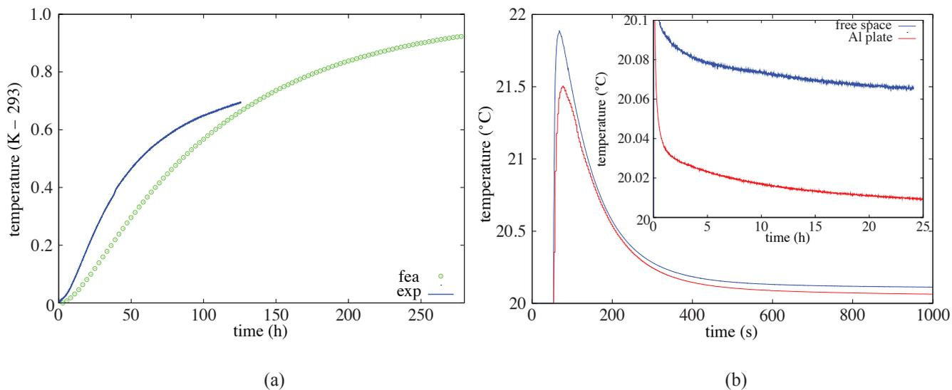
**Figure 4.** (a) The enclosure time constant was estimated to be 92 h experimentally and to be 116 h from finite element analysis. (b) Venting from high vacuum up to atmospheric air causes a large temperature jump with a short cooling time constant, but the small increase in equilibrium temperature takes much longer to settle.
