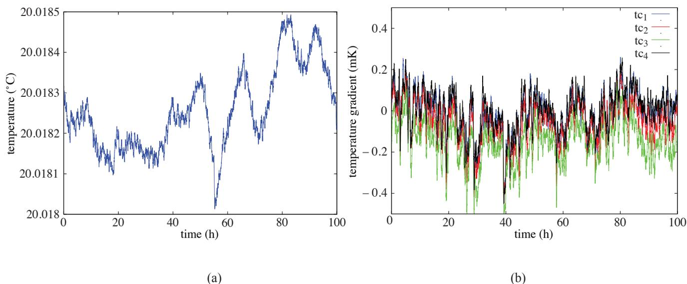
**Figure 5.** (a) Absolute temperature measured with a thermistor temperature standard remained stable to within 0.5 mK. (b) Gradients between the four thermocouples placed at the ends of the two cavities remained within 1 mK.
