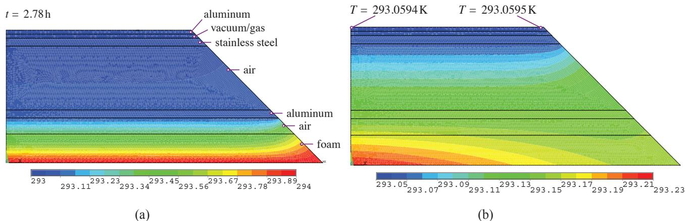
**Figure 3.** Finite element analysis was used to model (a) the time response of the passive thermal shielding and (b) steady state gradients arising from nonuniform room temperature outside the insulating foam.
