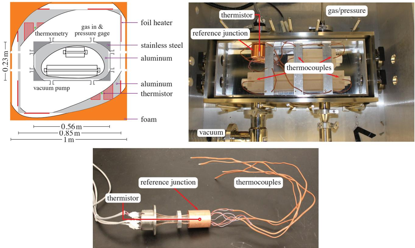
**Figure 2.** Temperature stabilization and thermometry configuration. Thermistors and foil heaters on the outer aluminum envelope were used to stabilize temperature. Thermocouples inside the vacuum chamber sensed temperature gradients around the optical cavities relative to a thermistor temperature standard.
