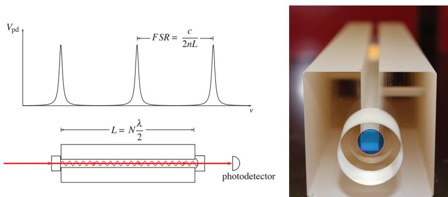
**Figure 1.** As a laser is swept in frequency, spikes of light intensity are observed at the output of the cavity when the laser achieves resonance. The frequency spacing between these intensity spikes is called the free spectral range.
