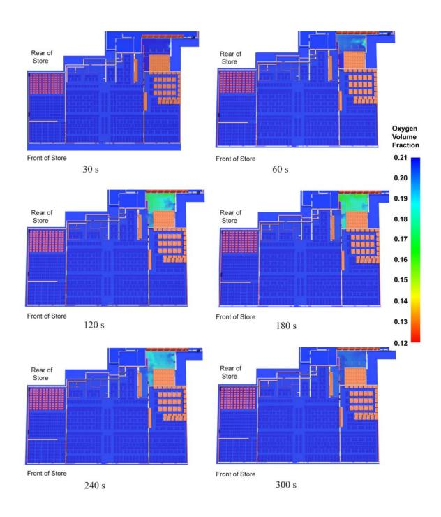
Figure K-45. Oxygen volume fractions 1.5 m (5 ft) above the floor in the sprinklered simulation.
