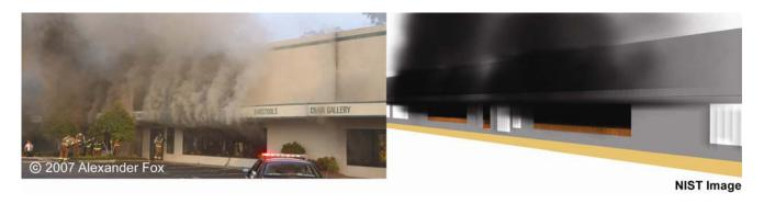
Figure K-24. Comparison between photo and rendered image from the simulation at 1530 s (7:36:23 p.m.). The view is of the front of the main showroom. Photo used with permission of Alexander Fox.
