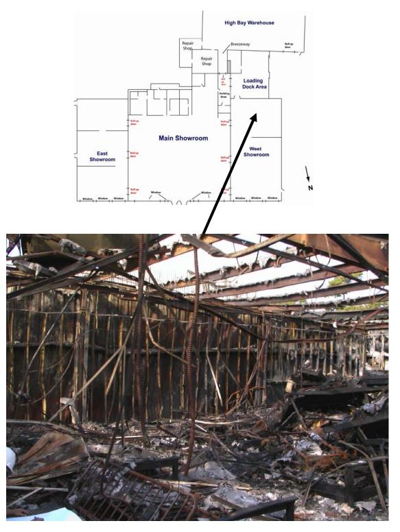
Figure E-23. Interior of rear portion of west showroom looking toward rear wall. Two tiered sofa and futon display shelves visible.
