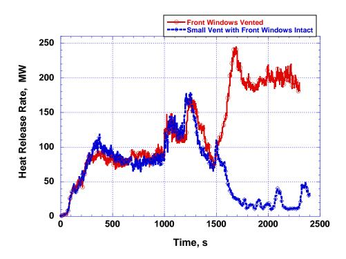
Figure K-61. Comparison of the heat release rate in the main and west showrooms between the base scenario and the scenario with the front windows intact and a small (1.69 m2) vent in the main showroom roof.
