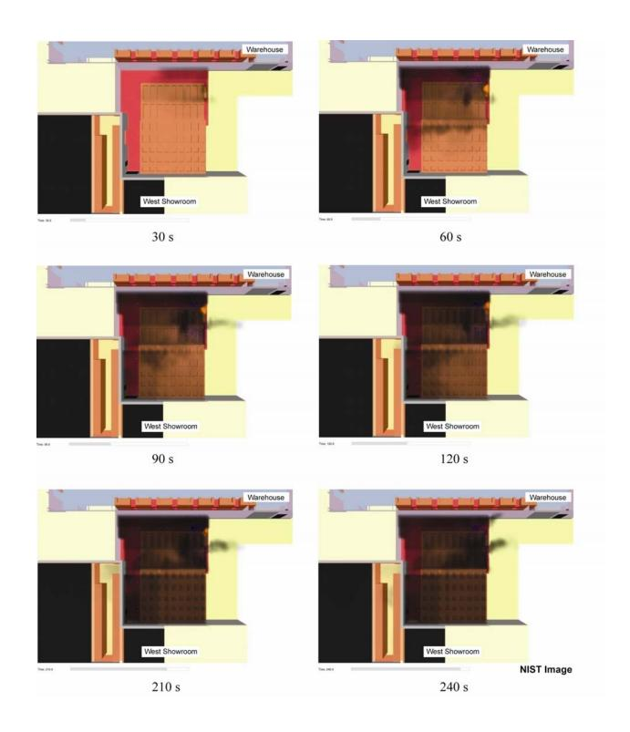
Figure K-42. Fire and smoke progression in the early stages of the sprinklered scenario. Sprinkler 3 was the first to activate, at 50 s, while sprinkler 6 activated at 75 s.
