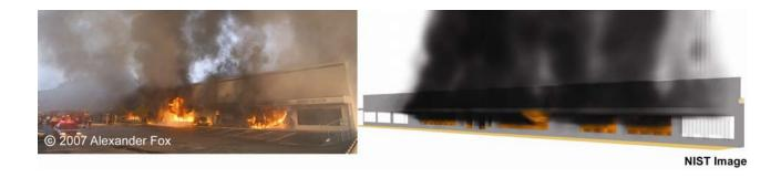
Figure K-27. Comparison between photo and rendered image from the simulation at 1884 s econds (7:42:17 p.m.). The view is of the front of the main and west showrooms. Photo used with permission of Alexander Fox.
