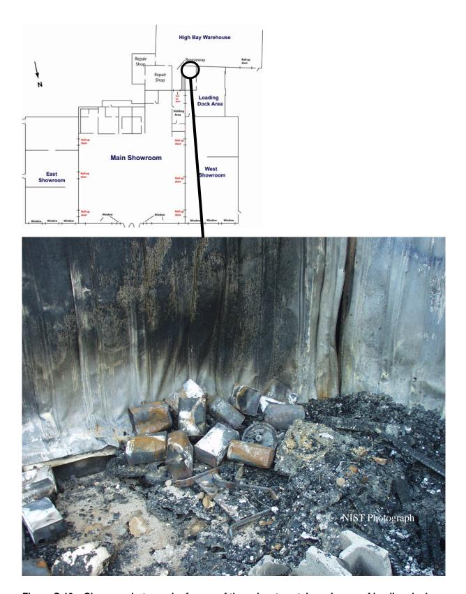
Figure C-19. Close up photograph of some of the solvent containers in rear of loading dock.
