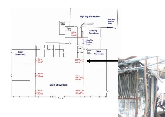
Figure O-29. Main showroom roll-up fire door looking toward rear of main showroom. Door identified as roll-up fire door #2 in Figure O-1.
