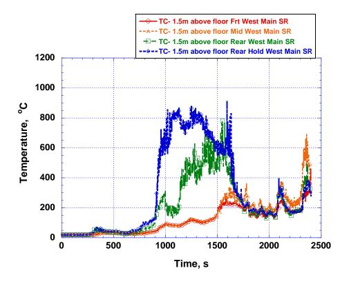
Figure K-64. West main showroom temperatures for 1.5 m (5 ft) above the floor.
