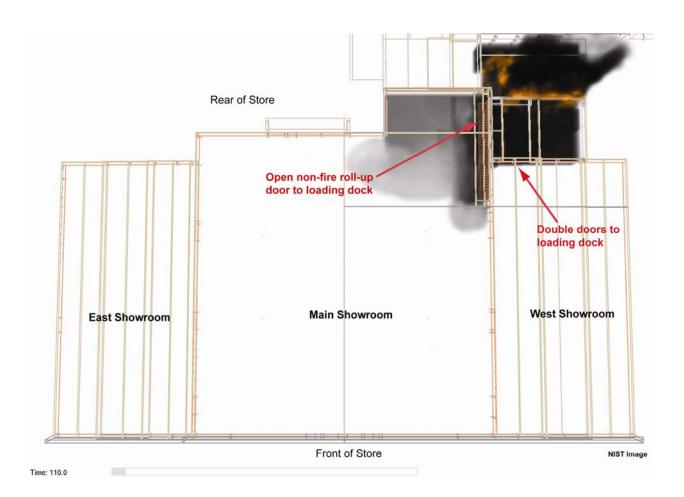
Figure K-14. Smoke filling in void space above main showroom. Image was rendered 110 s into the simulation.
