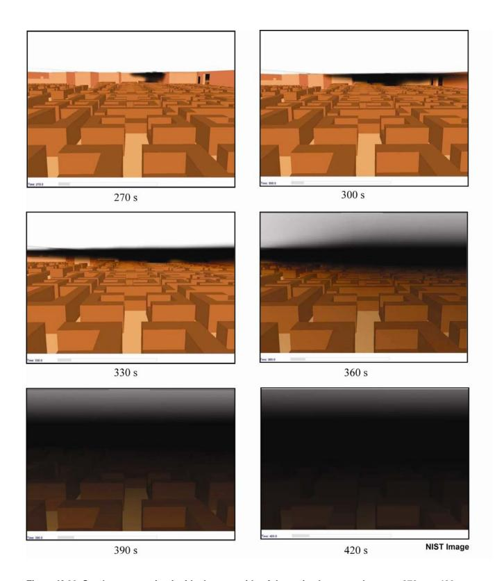
Figure K-20. Smoke progression inside the west side of the main showroom between 270 s to 420 s (7:15:23 p.m.).
