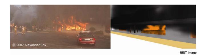
Figure K-25. Comparison between photo and rendered image from the simulation at 1655 s (7:38:28 p.m.). The view is of the front of the main showroom. Photo used with permission of Alexander Fox.
