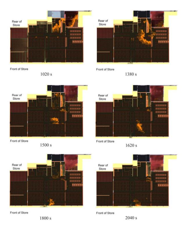
Figure K-46. Fire and smoke progression in case with front windows intact.
