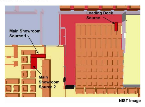
Figure K-10. Diagram showing locations of initiating fire sources in the loading dock and rear of main showroom.
