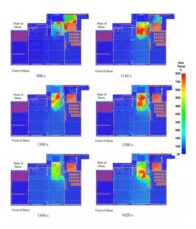
Figure K-75. Temperature slices located 1.5 m (5 ft) above the floor in simulation with front windows intact and large roof vent.
