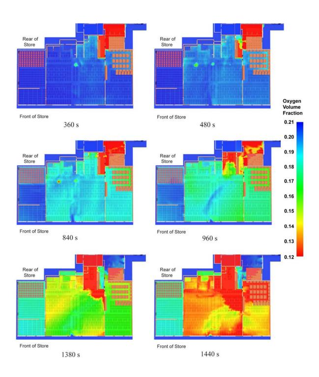
Figure K-67. Oxygen volume fractions (slice images) 1.5 m (5 ft) above the floor in simulation with front windows intact and small roof vent.
