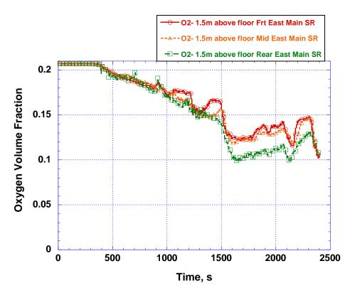
Figure K-71. East main showroom oxygen volume fractions for 1.5 m (5 ft) above the floor.
