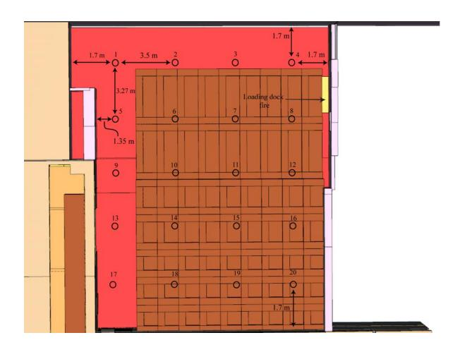
Figure K-41. Simulated sprinkler layout inside the enclosed loading dock.
