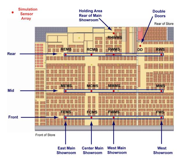
Figure K-29. Location of simulation sensor arrays in main and west showrooms.
