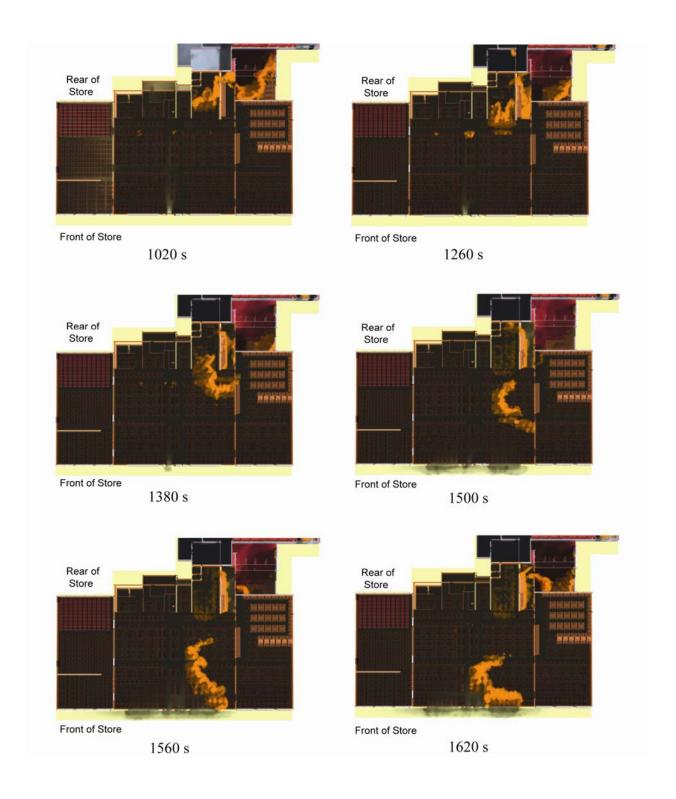
Figure K-22. View of fire (orange color indicates stoichiometric boundary) and smoke progression from above the showrooms from 1020 s to 1620 s (7:27:53 p.m. to 7:37:53 p.m.). The images are clipped to view conditions below the ceiling.
