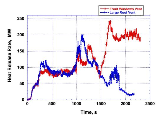
Figure K-74. Comparison of the heat release rate in the main and west showrooms between the base scenario and the scenario with the front windows intact and a large (5.91 m2) vent in the main showroom roof.
