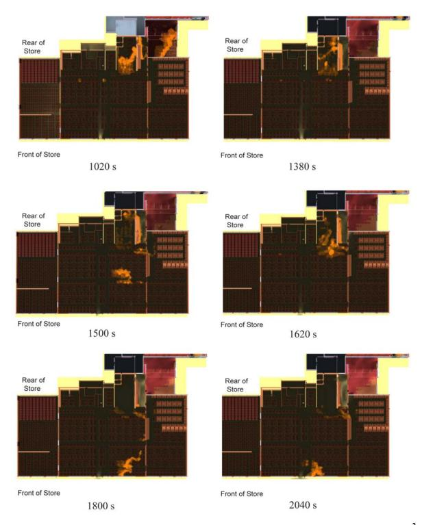
Figure K-73. Fire and smoke progression in scenario with front windows intact and large (5.9  $\mathrm{m}^2$ ) roof vent in showroom as rendered by computer simulation.
