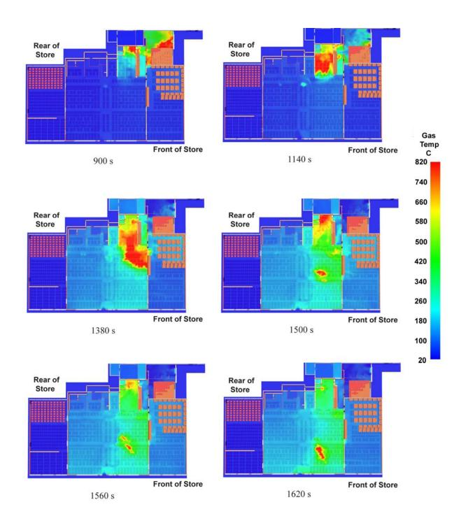
Figure K-48. Temperature slices located 1.5 m (5 ft) above the floor in simulation with front windows intact.
