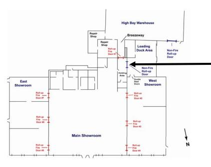
Figure O-11. Non-fire roll-up loading dock door looking toward rear of main showroom. Door was not designed as a fire door.
