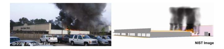
Figure K-23. Comparison between photo and rendered image from the simulation at 743 s (7:23:16 p.m.). The view is of the north west corner of the structure. Photo used with permission of Alexander Fox.
