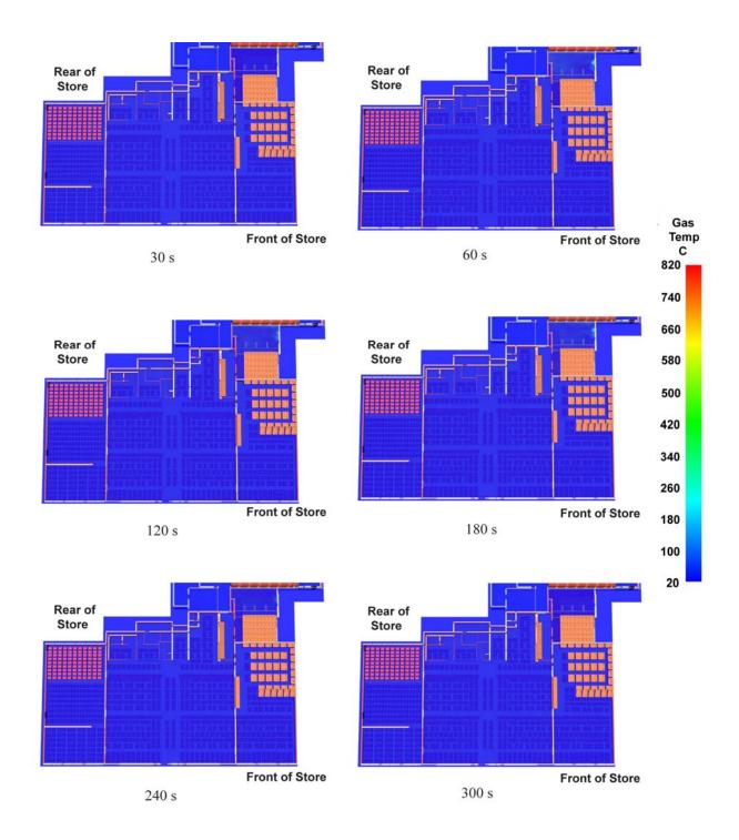
Figure K-44. Temperatures 1.5 m (5 ft) above the floor in the sprinklered simulation.
