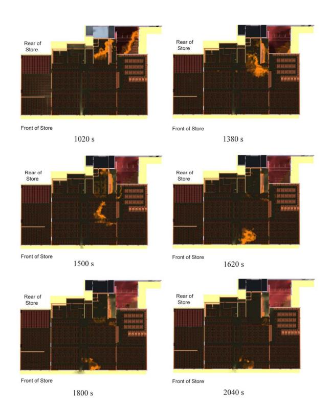
Figure K-60. Fire and smoke progression in scenario with front windows intact and small (1.69  $\rm m^2$ ) roof vent in showroom as rendered by computer simulation.
