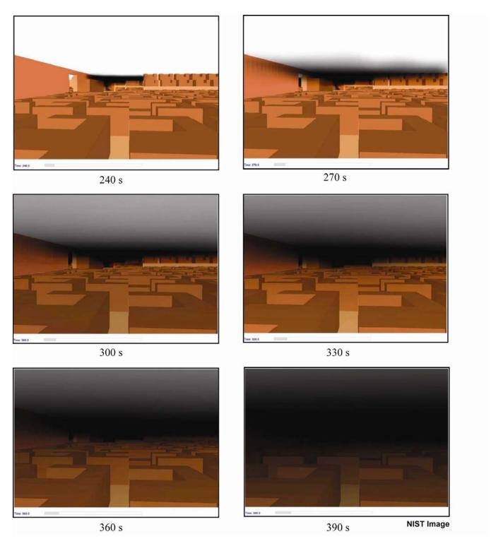
Figure K- 21. Smoke progression inside the west showroom between 240 s to 390 s (7:14:53p.m. to 7:17:23 p.m.).
