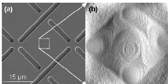
FIG. 1: SEM micrograph of the patterned surface and an AFM image ( $6\mu\text{m} \times 6\mu\text{m}$ ) taken after  $1200^\circ\text{C}$  flash heating inside one of the cells marked by the box. The atomic scale ordering of the steps are nearly identical in the center of each cell on.
