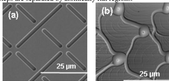
FIG. 3: (a) Scanning electron micrograph of the  $25\mu\text{m}$  square at  $45^\circ$  degrees. (b) Corresponding AFM image after  $1050^\circ\text{C}$  anneal of 18 hours. The current direction is from left to right.
