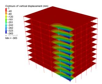
Figure 15. Peak vertical displacements of steel IMF building after dynamic removal of two columns.
