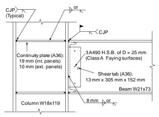
Figure 1. WUF-B connection details for the steel assembly.
