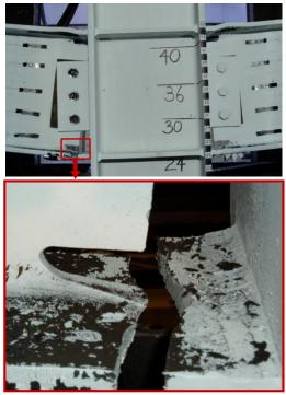
Figure 4. Failure mode of the steel assembly.
