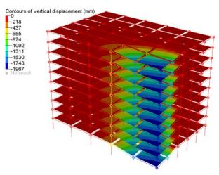
Figure 17. Vertical displacements from pushdown analysis of concrete IMF building with three missing columns.
