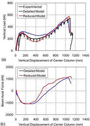
Figure 11. Vertical load and beam axial force versus vertical displacement of center column for the reinforced concrete assembly (measurement uncertainty  $\pm 1$  %).
