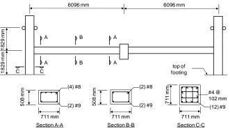
Figure 8. Schematic of the reinforced concrete assembly.
