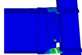
Figure 7. Failure mode from detailed model of the steel assembly.
