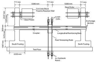
Figure 9. Test setup for the reinforced concrete assembly.
