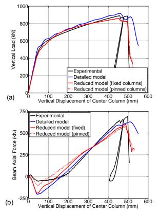
Figure 5. (a) Vertical load and (b) beam axial force versus vertical displacement of center column for the steel assembly (measurement uncertainty:  $\pm 1$  %).
