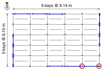
Figure 16. Plan layout for steel IMF building. Perimeter moment frames shown in heavy blue lines; circles indicate columns removed dynamically under service loads.
