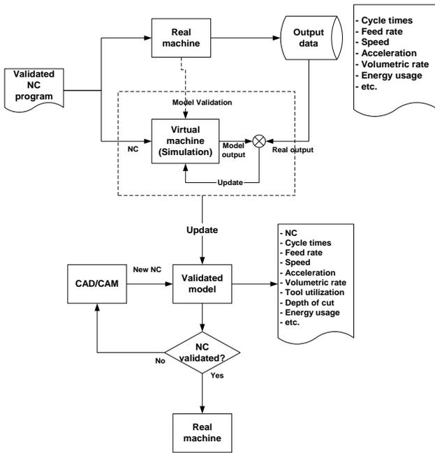
Figure 1. Virtual machine model validation methodology
