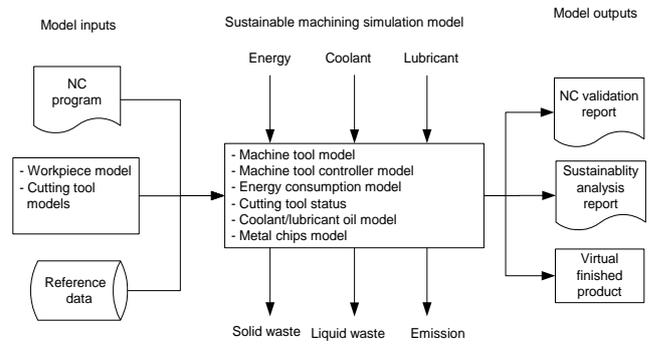
Figure 2: Overview of sustainable machining simulation model
