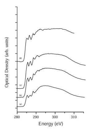
Figure 4: Carbon XANES spectra from coal samples showing the affects of varied voltage under cryogenic conditions: a) "pristine" microtomed sample, b) cryo-FIB section with 5 kV and 2 kV final polishing, c) cryo-FIB section with a 30 kV final polish, d) FIB sample with a 500 V final polish in a Fischione Nanomill at liquid nitrogen temperature. None of these samples were exposed to an electron beam.
