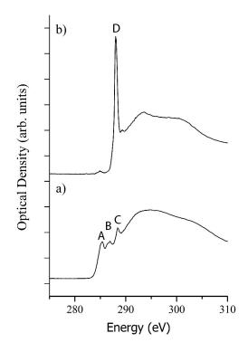
Figure 1: Carbon K XANES Spectra from microtomed samples: a) lignite coal and b) PAAm. Uppercase letters denote  $1s \rightarrow \pi^*$  photoabsorption peaks corresponding to A) aromatic (or olefinic) C=C at 285.2 eV, B) Aromatic ketone C<sub>aromatic</sub>-C=O at 286.6 eV, C) carboxyl carbonyl - (C=O)OH at 288.5 eV, D) Amide NH<sub>2</sub>-C=O at 288.0 eV functional groups.
