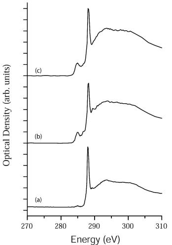
Figure 8: Carbon XANES spectra of PAAm prepared with various values of ion beam overlap: a) pristine microtome section, b) sample processed with 0% beam overlap, and c) sample processed with 50 % beam overlap (previously shown in Figure 5D). The final milling steps for the FIB sections were prepared without SEM imaging and a final ion current of 30 pA.
