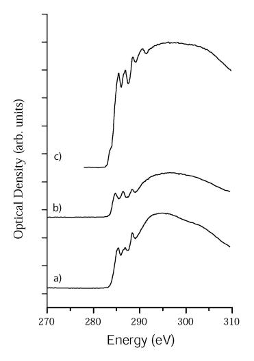
Fig 2: Comparison of a) microtomed coal, b) FIB-prepared coal with a 30 kV final ion polish with 5 keV electron beam irradiation, and c) FIB-prepared coal with a 30 kV final polish with no electron beam irradiation.
