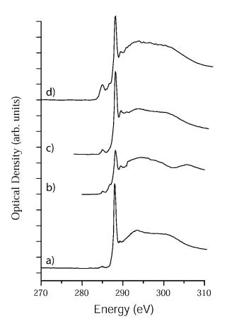
Figure 5: Carbon XANES spectra of PAAm showing the effect varying final polishing voltage: a) "pristine" microtomed sample, b) FIB-prepared sample with a 1 kV final polish, c) FIBprepared sample with a two-step (5 kV and 2 kV) final polish, d) FIB-prepared sample with a "standard" 30 kV final polishing voltage. All samples have been prepared without visualizing with the electron beam.
