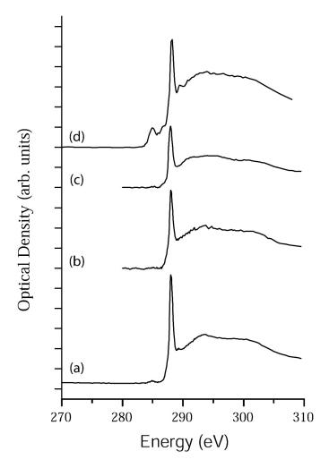
Figure 6: XANES data from microtomed PAAm that had been heated to various temperatures : a) unheated PAAm; b) sample that had been vacuum annealed at 128 °C, c) sample that had been annealed at 231 °C; d) FIB-prepared PAAm with no SEM imaging (previously shown in Figure 5d) and 30 keV final thinning voltage.
