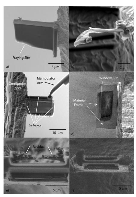
Figure 7: Effects and mitigation of sample softening in the FIB. a) Side view of a PAAm section that is beginning to degrade and warp b) Top view of the same section after additional FIB milling. Section rigidity may be maintained by either a c) Pt frame configuration or a d) natural frame surrounding the section. Top views of sections supported by e) a Pt Frame and f) a natural frame.
